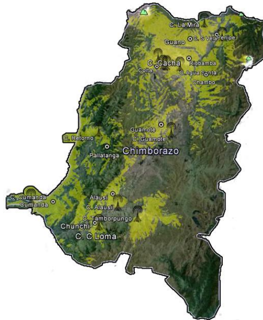
Figura 5. Cobertura UL DVB-RCT2 MODCOD QPSK \frac{1}{2} .
