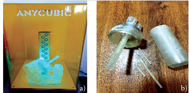
Figure 4. Bioreactor design for mesenchymal stem cells printed: a) curing the model inside the Anycubic printer with UV light and b) the printed model.
