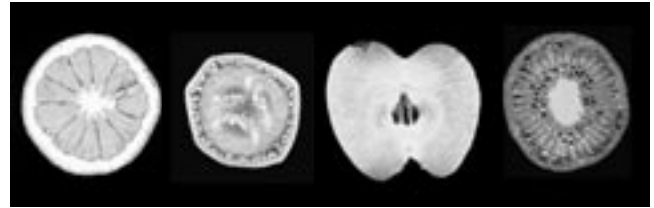
Figure 1. 2D MRI sections obtained from different intact fruits using a conventional spin-echo (SE) pulse sequence. Starting from left: an orange, a banana, an apple and a kiwi.
